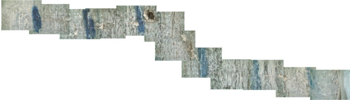
Figure F.9: Microscopy image (6.3x zoom) of T3-F15 flexure crack
