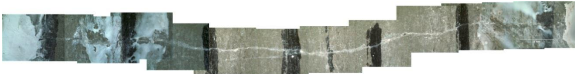
Figure F.8: Microscopy image (6.3x zoom) of Type II tension crack
