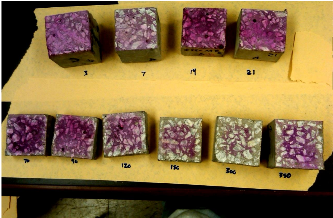
Figure D.4: F25-MK5 carbonation samples (76.2 x 76.2 mm (3 x 3 in.))
