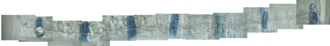
Figure F.10: Microscopy image (6.3x zoom) of T3-F15 tension crack
