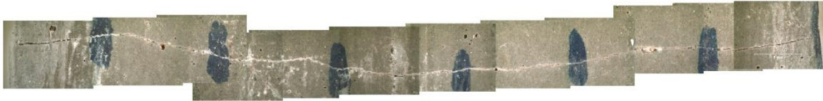
Figure F.16: Microscopy image (6.3x zoom) of S50-MK5 tension crack
