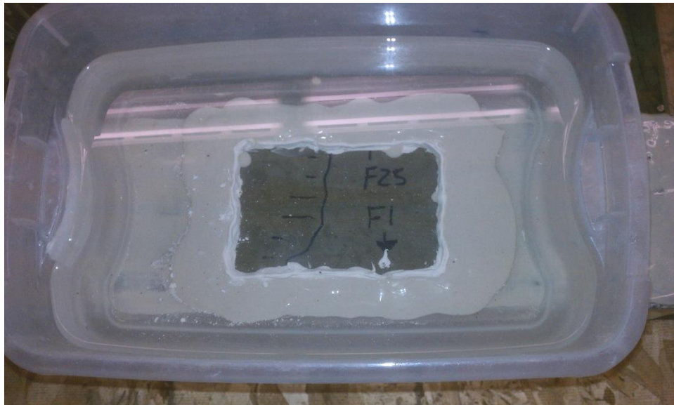
Figure F.6: Exposure surface inside of ponding container with simulated seawater solution
