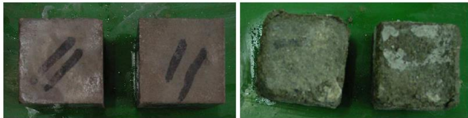
Figure 2.17: 10% silica fume mortars exposed to 5% sodium sulfate (left) and 5% magnesium sulfate (right) (Lee, et al., 2005)
