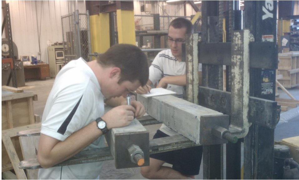
Figure F.3: Graduate students taking crack width measurements before sealing and exposure
