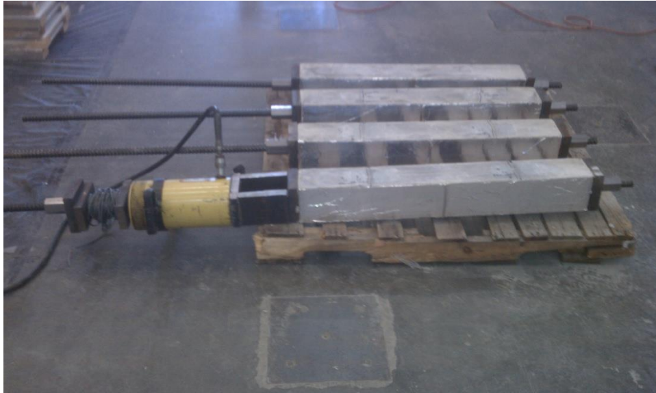
Figure F.1: Post-tensioning of specimens
