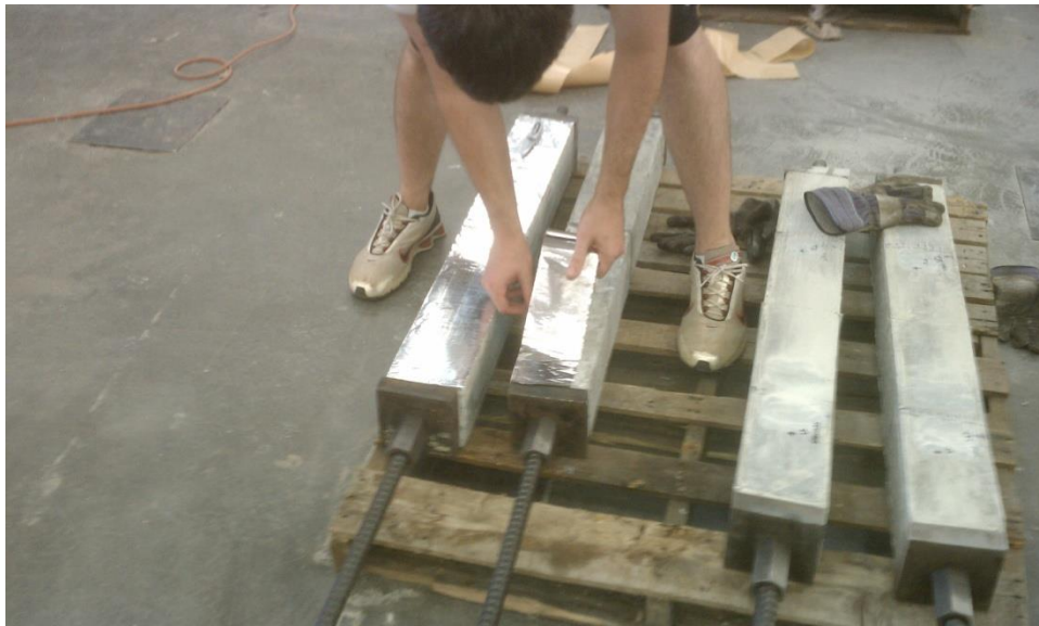
Figure F.4: Graduate student sealing the sides of specimens with aluminum tape
