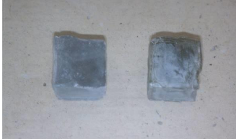
Figure 6.4: T5 control sample (left) and 180 day exposure specimen (right)
