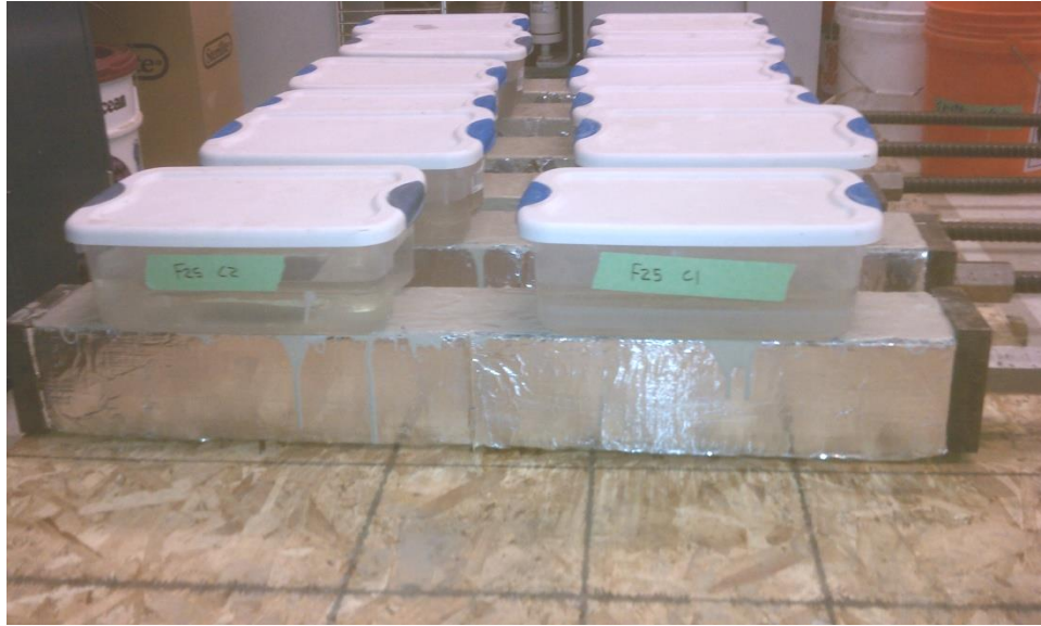
Figure F.5: Sealed specimens with aluminum tape and epoxy with exposure container attached
