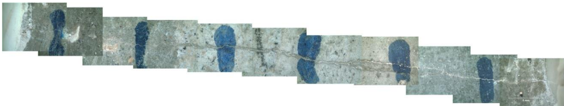
Figure F.13: Microscopy image (6.3x zoom) of S35-MK5 flexure crack
